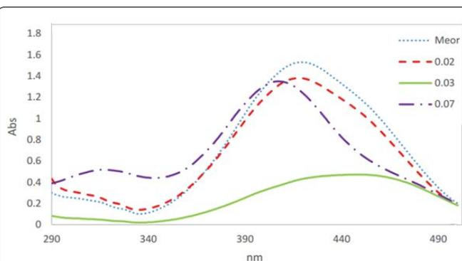
Figure 5: Effect of TiO<sub>2</sub>/(HPA/DAZY) ratio on the photodegradation of MO. Concentration of methyl orange was  $5.0 \times 10^{-5}$  M.
