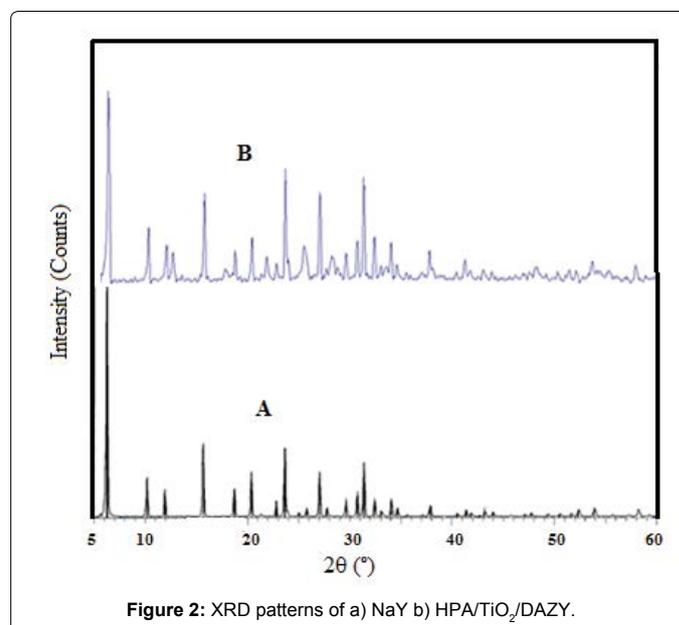
Figure 2: XRD patterns of a) NaY b) HPA/ $TiO_2$ /DAZY.
