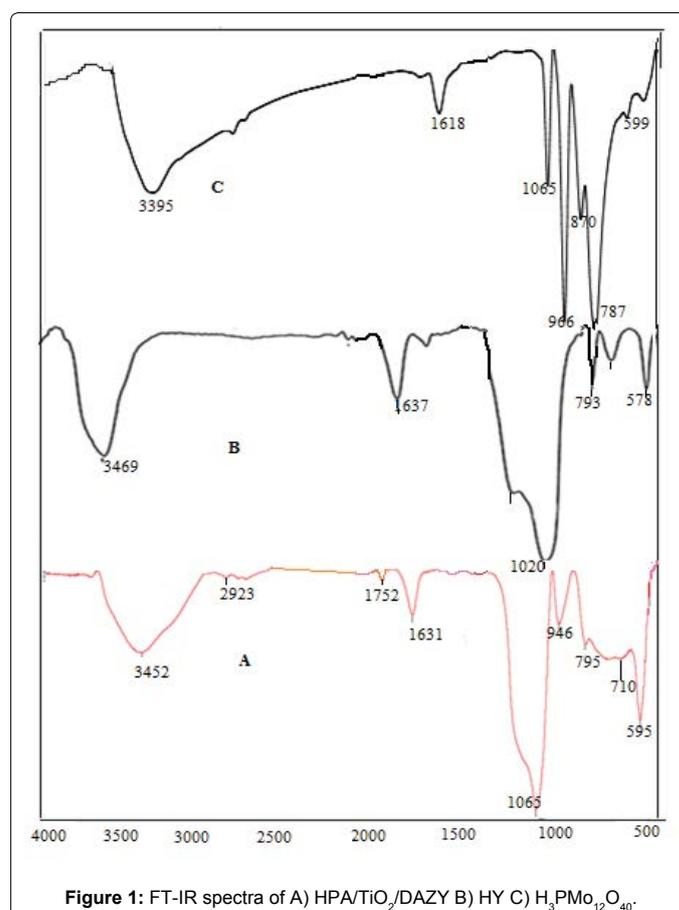
Figure 1: FT-IR spectra of A) HPA/ $TiO_2$ /DAZY B) HY C)  $H_3PMO_{12}O_{40}$ .
