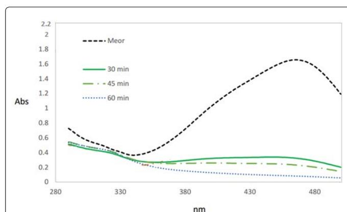
Figure 7: Absorption spectral changes of the filtered solution of methyl orange after irradiation in the presence of HPA/TiO<sub>2</sub>/HY. Concentration of methyl orange was  $5.0 \times 10^{-5}$  M.
