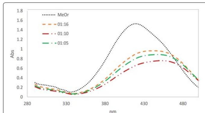
Figure 6: Effect of catalyst amount on the photodegradation of MO. Concentration of methyl orange was  $5.0 \times 10^{-5}$  M.
