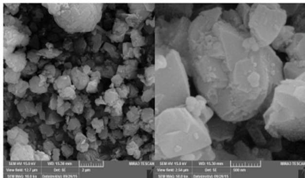
Figure 3: FESEM micrograph of HPA/TiO<sub>2</sub>/DAZY.
