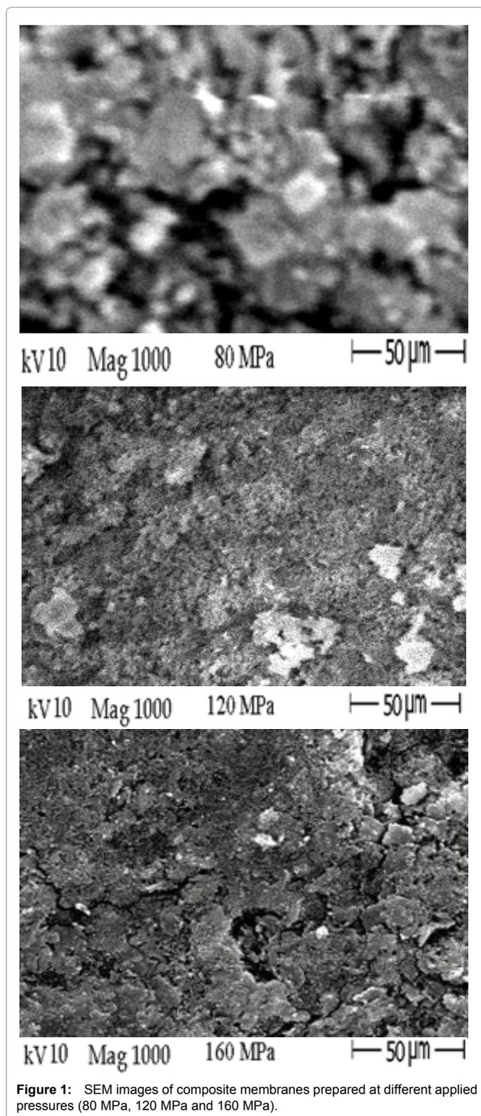
Figure 1: SEM images of composite membranes prepared at different applied pressures (80 MPa, 120 MPa and 160 MPa).
