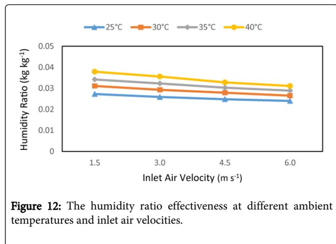
Figure 12: The humidity ratio effectiveness at different ambient temperatures and inlet air velocities.
