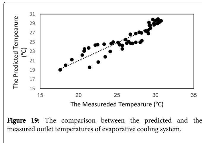
**Figure 19:** The comparison between the predicted and the measured outlet temperatures of evaporative cooling system.
