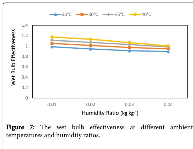
**Figure 7:** The wet bulb effectiveness at different ambient temperatures and humidity ratios.
