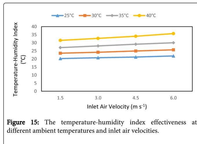
Figure 15: The temperature-humidity index effectiveness at different ambient temperatures and inlet air velocities.
