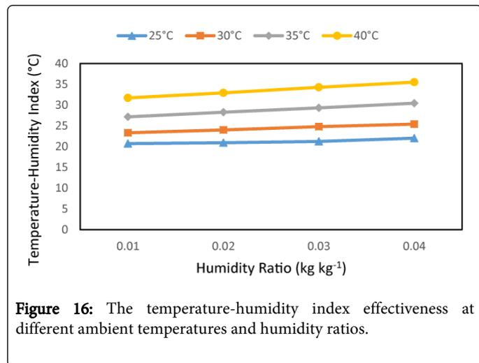
**Figure 16:** The temperature-humidity index effectiveness at different ambient temperatures and humidity ratios.
