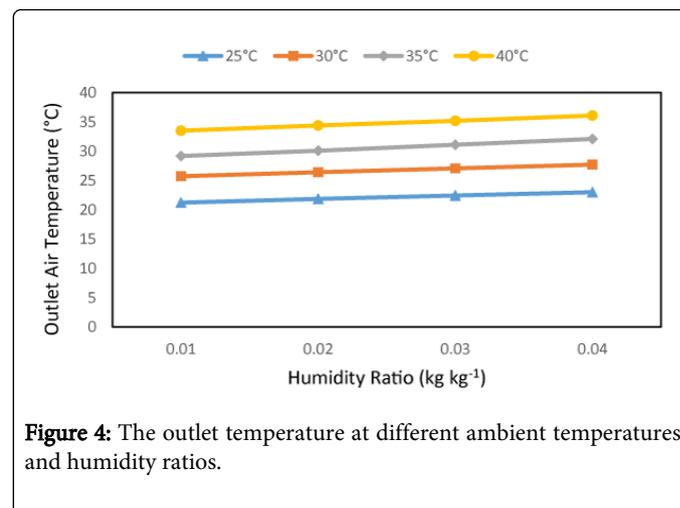
Figure 4: The outlet temperature at different ambient temperatures and humidity ratios.
