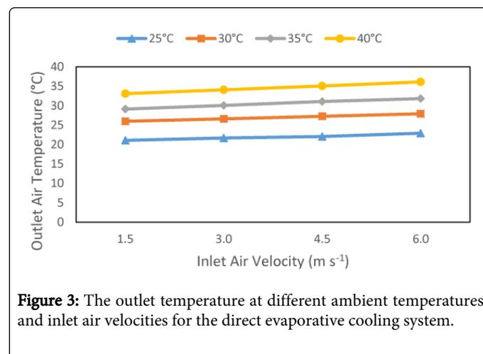
Figure 3: The outlet temperature at different ambient temperatures and inlet air velocities for the direct evaporative cooling system.
