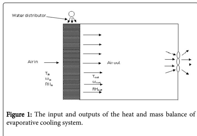
**Figure 1:** The input and outputs of the heat and mass balance of evaporative cooling system.
