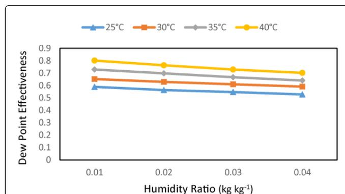
**Figure 10:** The dew point effectiveness at different ambient temperatures and humidity ratios.
