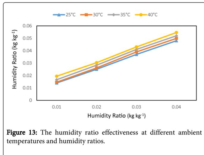
Figure 13: The humidity ratio effectiveness at different ambient temperatures and humidity ratios.
