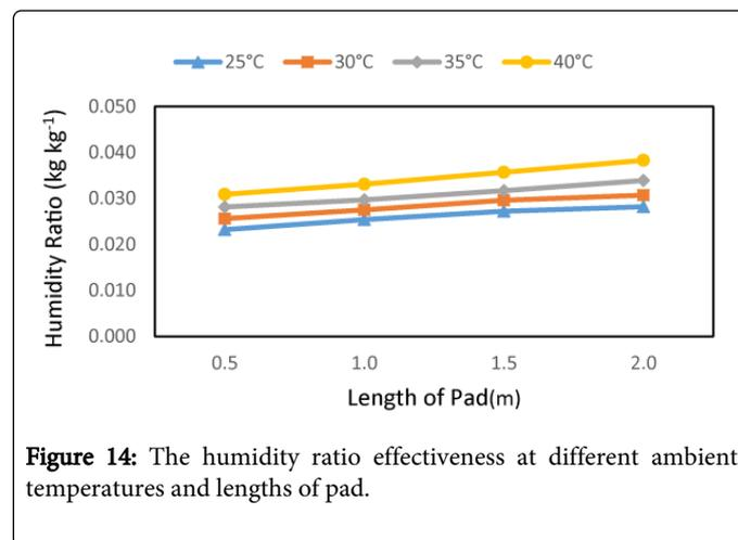
Figure 14: The humidity ratio effectiveness at different ambient temperatures and lengths of pad.
