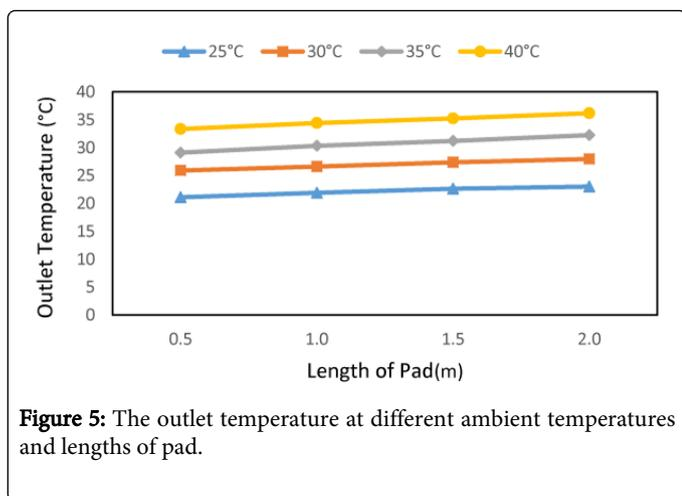
**Figure 5:** The outlet temperature at different ambient temperatures and lengths of pad.
