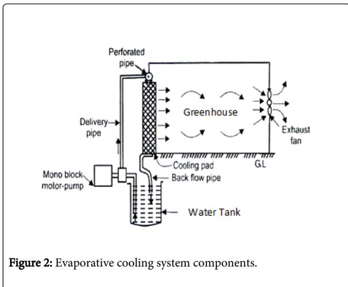
Figure 2: Evaporative cooling system components.
