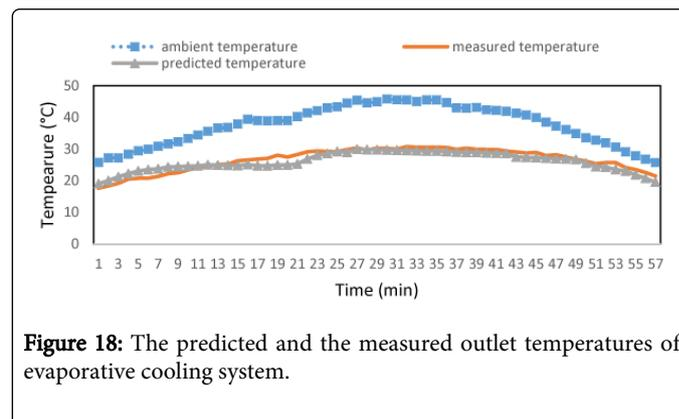
**Figure 18:** The predicted and the measured outlet temperatures of evaporative cooling system.
