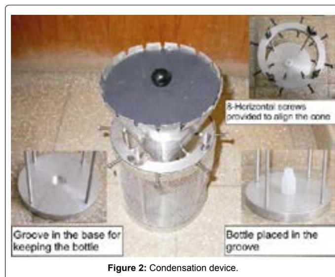
cone can fall straight into the bottle and the falling droplets can be seen. Depending on prevalent relative humidity, it takes 30 minutes to 60 minutes for collecting 5 to 10 ml of liquid condensate. However, during the rainy season when relative humidity is very high, the sampling bottle is filled even within 30 minutes. After setting up the conical condensation device the date, time, temperature and relative humidity are recorded using thermo-hygrometer [29].
