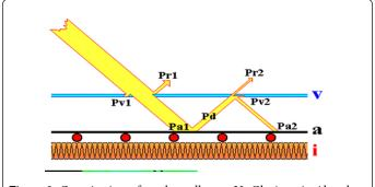
**Figure 2:** Constitution of a solar collector. V=Glazing. A=Absorber. I=Thermal insulation. Creation of the greenhouse effect.
