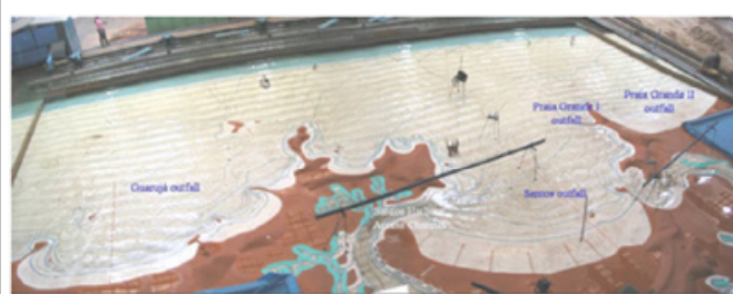
Figure 6: Scale model of Santos Bay, Estuary and Harbor and nearby beaches
